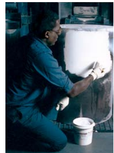
Figure 4 Water-based coating used to protect graphite from oxidation.
