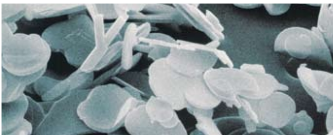
Figure 1 Typical (h)BN powder. Flat platey crystals about 10µm.
